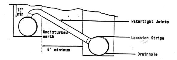
NOTE: Invert of the septic tank outlet shall be at least one inch higher than the top of the gravelless pipe.
